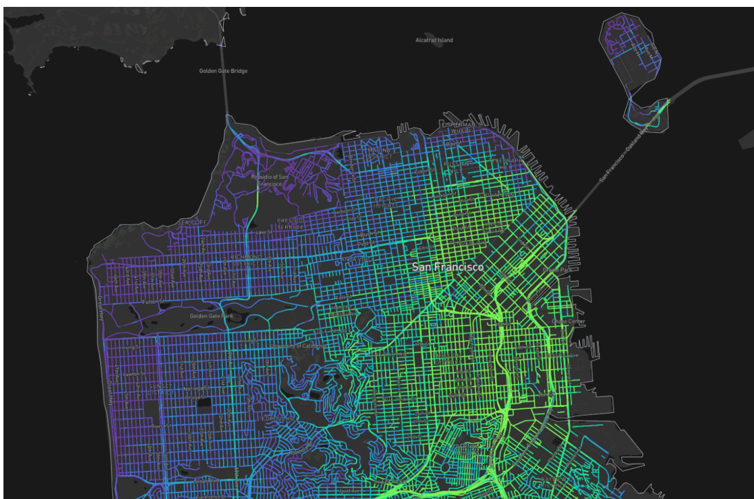
Figure 2: Example of plotted ambient concentration estimates for NO 2 in the San Francisco Bay Area, CA. This plot uses data generated by the broad area monitoring method.
